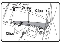
1: Park wipers straight up. Open bonnet. Remove screw cover. Remove screw. Lift 2 clips at rear. Undo 3 clips at front & lift cover out.
