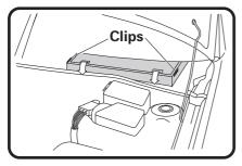
2: Release clips & fold front down to remove filter.
